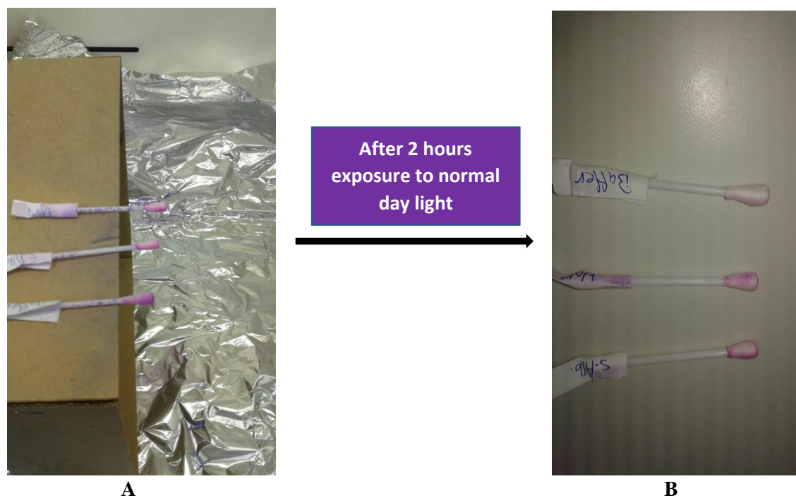
Figure 4 A) illustrate when we took 3 swabs and immerse them on stock DNA, Buffer and BSA then sprayed by DODC. B) showed the effect of normal day light after 2 hours.
