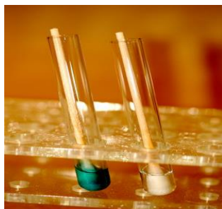
Figure 9 The image shows a positive BCIP test on the left and a negative test on the right.
