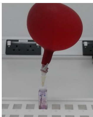
Figure 4.11 balloon full of N 2 to deoxygenate the buffer.
